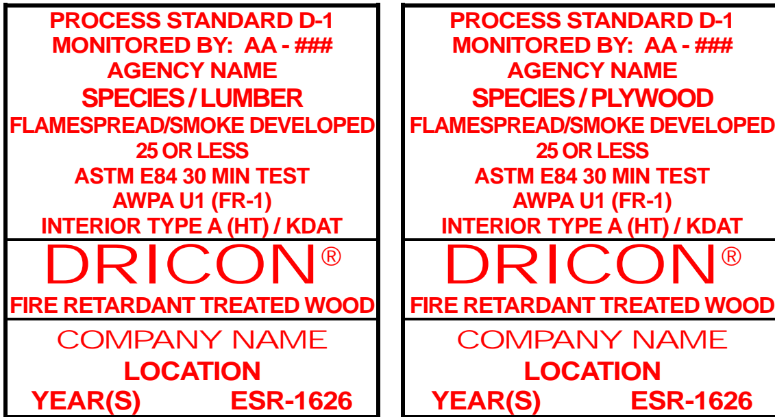
FIGURE 1—LUMBER AND PLYWOOD STAMPS 1,2,3
